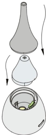
5. Replace the water tank cover and then the outer cover, ensuring they are securely in place.
