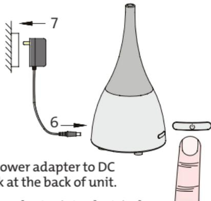
6. Connect power adapter to DC power jack at the back of unit.
