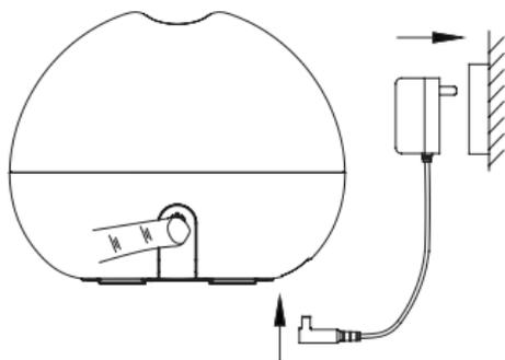
5. Connect power adapter to DC power jack on bottom side of unit.
