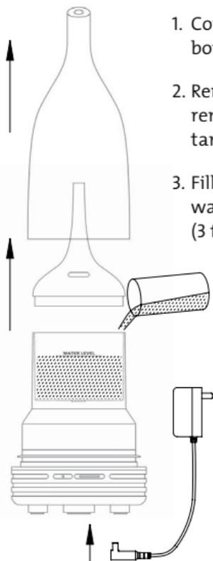
1. Connect power adapter to DC power jack on bottom of unit.
