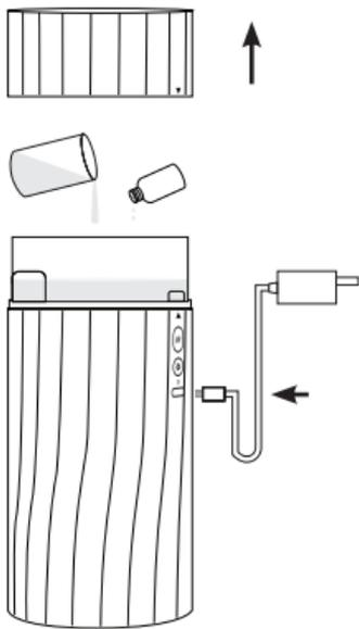
5. Replace the cover. Ensure the arrow indicator on the cover and base are lined up. Rotate the upper cover to align. Unit will not turn on if the top arrow does not line up with the lock icon.
