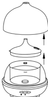
2. Remove the ceramic cover from the base, then remove the water tank cover from the water tank.
