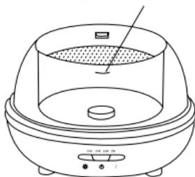
3. Fill water tank with room temperature tap water to no higher than max. water level line (15 fl. oz./450 ml).
