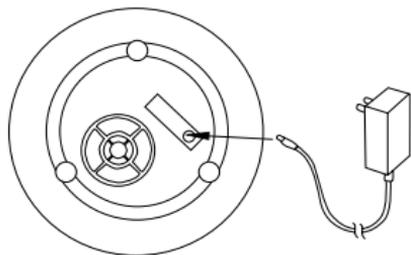
1. Connect power adapter to DC power jack on bottom of unit.
