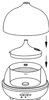
5. Replace the water tank cover and then the ceramic cover; ensure that the ceramic cover is pressed down over the silicone o-ring.
