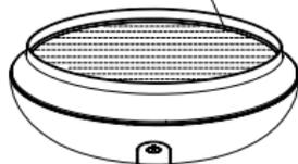
2. Using the measuring cup provided, fill water tank with room temperature tap water to no higher than max. water level line (6 fl oz/180 ml).
