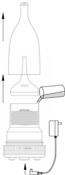
1. Connect power adapter to DC power jack on bottom of the unit
