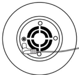
1. Connect power adapter to DC power jack on bottom of unit before filling the water tank with water.
